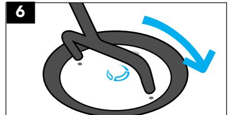
Insert new cartridge into housing and turn key to right (clockwise) to lock and click into place.
