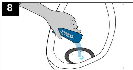
Add blue sealant (allow time to drain into cartridge).
