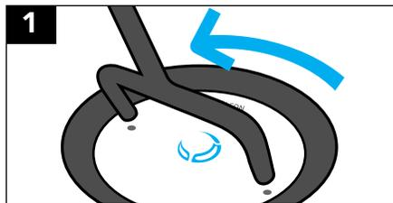
Insert Key into cartridge, turn key to left to unlock.
