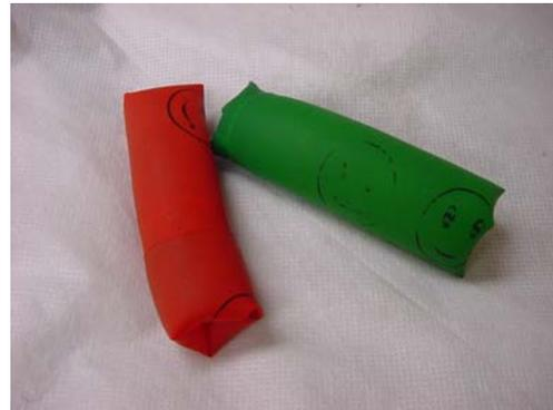
Although not exact, the green specimen (160g) was compared to a media mass loading of 150g, and both the green and red specimens combined (292g) was compared to a media mass loading of 300g. Testing was completed on three different toilet types: rim-jet gravity model, 4-L pressure-assist model, and washdown model. Test results are illustrated in Figures 16a and 16b.
