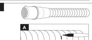
**A. Find the drain nipple depth** on the Tube Cutting Chart (left). **Measure and mark the specified trim length** on the insert tube at the nearest 1/4" groove.
