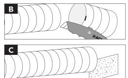
B. Cut the tube at the groove using a sharp utility knife to ensure a square, flat cut.C. Clean burrs from the cut end by using emery paper.
