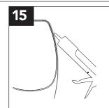
**CAULK THE BOWL TO THE WALL** if there is good flow and no leaks or standing water.
