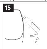
**CAULK THE BOWL TO THE WALL** if there is good flow and no leaks or standing water.
