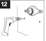
**DRILL HOLES** with 5/16" masonry bit for the lower anchor screws and insert plastic anchors.
