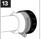
**TIGHTEN COMPRESSION NUT AND GEAR** CLAMP.
