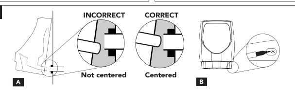
A. Hang the bowl on the bracket and check tail pipe alignment, then remove the bowl and adjust the bracket as needed.
