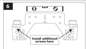
LEVEL THE BRACKET THEN MARK, drill and install two additional plastic anchors and screws. If preexisting bearing rods can be used, screws are not necessary.
