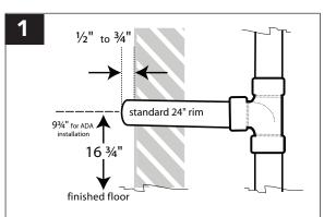
SET DRAIN LINE HEIGHT 16 ¾" from finished floor (standard 24" rim) or 934" for ADA installation. Threaded nipple should extend ½ to ¾" from wall.
