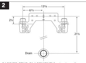
**CARRIER STUD PLACEMENT** If using in-wall carrier, set bearing rods as shown above.
