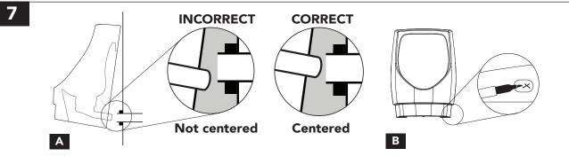
A. Hang the bowl on the bracket and check tail pipe alignment, then remove the bowl and adjust the bracket as needed. Re-hang and re-check bowl alignment with the drain line. Tail pipe should align with center of drain line.
