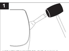
**USE UTILITY KNIFE TO CUT CAULK** then use a putty knife and mallet to remove the bowl. Remove hanger brackets, scrape off caulk, and clean the wall.
