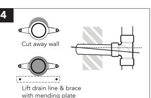
**ADJUST DRAIN TO ACHIEVE PITCH** only if standing water is present (code requires ¼ "drop per foot of drain line for proper pitch). Seal wall
