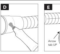
**D. Apply lubricant** to the outside of the rubber bushing and ribbed inside area.
