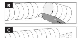
**B. Cut the tube** at the groove using a sharp utility knife to ensure a square, flat cut.
