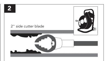
**IMPORTANT:** Use a drain machine to remove build-up inside pipes. Clean up to 25 feet deep then flush with water to remove cutting debris. **Never install on copper DWV.**
