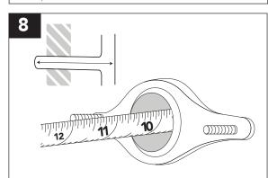
**DETERMINE THE DRAIN NIPPLE DEPTH** by measuring the distance between the back of the sanitary tee (or elbow) to the front edge of the nipple.
