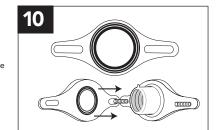
PLACE THE SEAL INTO THE FLANGE with the ribs facing out. Install the flange with washers and hex nuts, but do not tighten completely.
