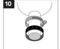
PLACE THE GEAR CLAMP and compression nut onto the housing tailpipe.
